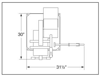
Figure 5. Minimum working clearances.
